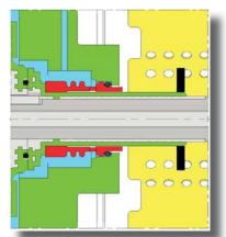
Single internal mechanical seal for applications with clean fluids or low to moderate contaminated, such as CRANE 2N
