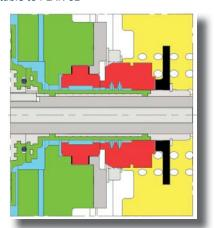
Single external mechanical seals, with PTFE bellow, suitable for corosive fluids without solid parts, such as CRANE10T
