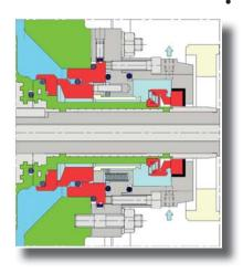
In case of liquid cristallization, due to air contact, CDR offers plan 62.
