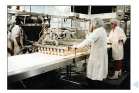
A leading designer and manufacturer of machinery for producing savoury pies, pasties and sausage rolls is incorporating stainless steel W032 pumps into its sausage roll manufacturing machines. Transferring prepared sausage meat in a continuous uniform length to the pastry casing at a capacity of between 5-10m<sup>3</sup>/h, the W range features an auger feeding system to ensure the sausage meat is consistently fed from the extended hopper inlet to the pumping element.
