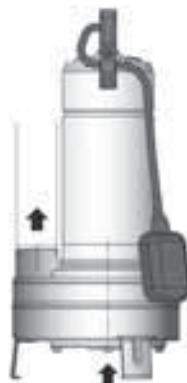
Pump with pipe screwed into the delivery port
