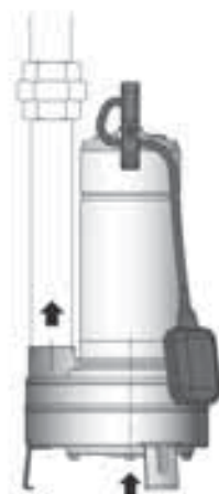
Pump with pipe and union (locally available)
