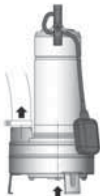
Pump with hosetail seat and clamp (locally available)
