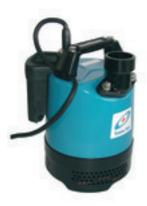
Handles like a non-automatic pump - no special installation procedures. Sensitive electrodes detect water to start up pump operation even when foreign matters are present. Relay sensor completely molded in resin and covered by rubber case for protection against rough handling.
