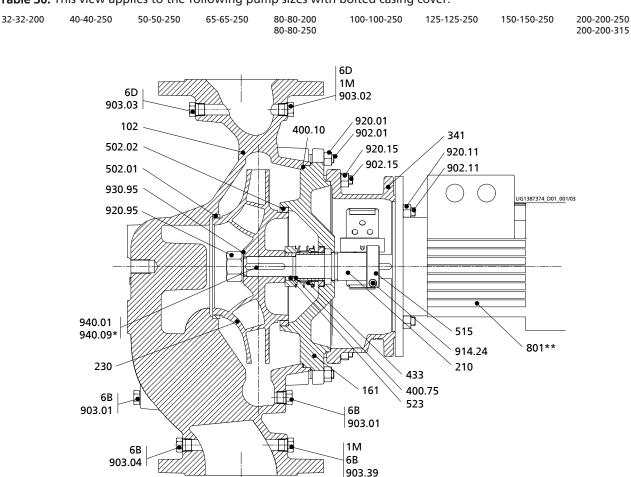
General assembly drawing, \* Second key only for WS 55; \*\* With motor foot from motor size 132
