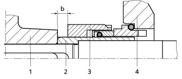
Fig. 8: Installation dimension b of mechanical seal
