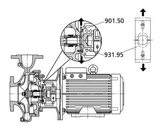
Fig. 10: Removing the lock washers
