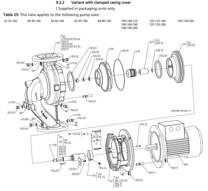
**Fig. 12:** Pump set with single mechanical seal and clamped casing cover **Table 26:** List of components
