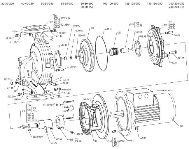
Fig. 11: Variant with bolted casing cover
