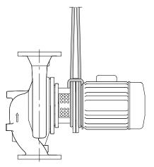
Fig. 1: Transporting the pump set
