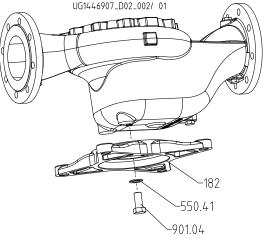
Fig. 14: Vertical installation with pump foot Table 29: List of components
