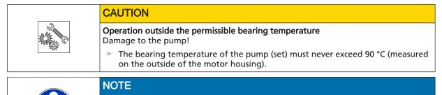
After commissioning, increased temperatures may occur at grease-lubricated rolling element bearings due to the running-in process. The final bearing temperature is only reached after a certain period of operation (up to 48 hours depending on the conditions).
