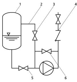
Fig. 7: Vacuum balance system
